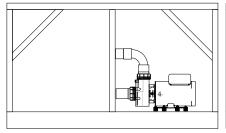
Microsilk Pump location on right side of spa when standing at the control panel
