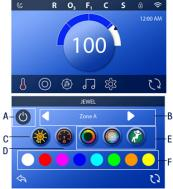
(C) Dimmer Control: Pressing repeatedly will dim the brightness of the lights until they are off. Pressing again will start the cycle over.
