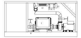
Auxiliary Pump location on left side of spa when standing at the control panel
