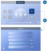
There are two types of filters: Low Pass and High Pass. These filters apply to the rear speaker output only. Select Low Pass for subwoofers or High Pass for tweeters. Select OFF if filtering is not desired. Regular speakers do not require filtering.
